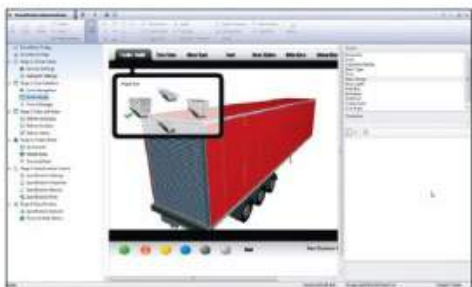
3 In DriveWorks Administrator build the interface (forms) and rules to drive how your model will change
